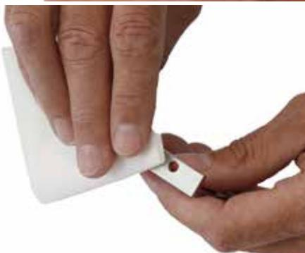
Dry the bracket thoroughly before applying the glue.
