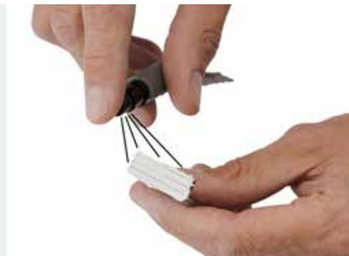
Use the hand spray to activate the glue by spraying the fluid directly on the glue.
