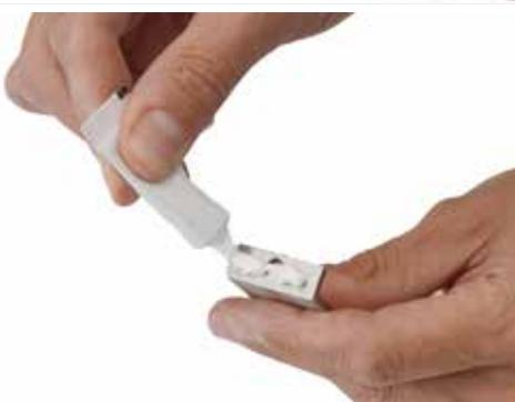
Apply the glue in a layer approximately 3-5mm thick.
