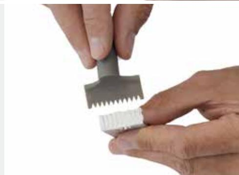
Drag the "rake" across the glue and fluid a couple of times to ensure that the two materials are mixed together.
