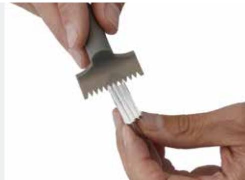
Using the small "rake", drag tracks through the glue.
